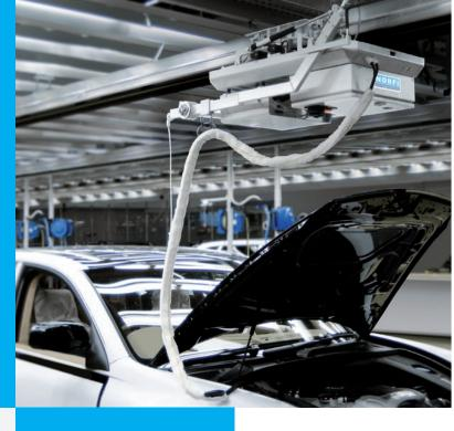
In car production lines, it often is necessary to charge the batteries of the vehicles. Otherwise, the cars are leaving the finish lines with only partly charged batteries and have to be taken to rectification areas where they then are connected to stationary chargers. Charging the batteries along the finish lines helps to avoid this additional work.
