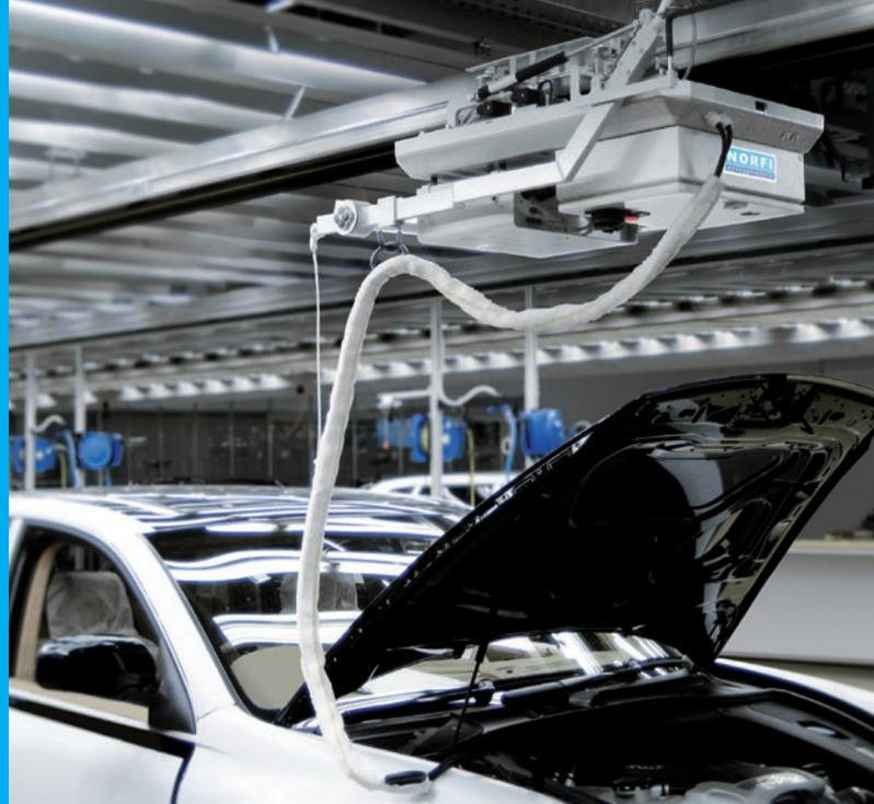
*In car production lines, it often is necessary to charge the batteries of the vehicles. Otherwise, the cars are leaving the finish lines with only partly charged batteries and have to be taken to rectification areas where they then are connected to stationary chargers. Charging the batteries along the finish lines helps to avoid this additional work.*
